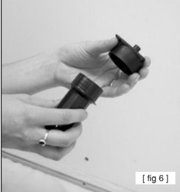
Assemble adjustable leg by attaching the dowel head to the leg (fig. 6, 6A, and 6B). Take the assembled leg and insert dowel into the hole provided as in fig. 6A. Use 1/2" screws and screw leg into bottom of cabinet to keep it firmly in place (fig. 6C and 6D). Let glue dry
